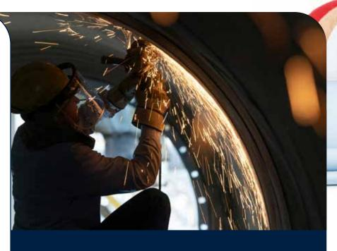
The range of possible applications for our abrasives varies with grit size from coarse sanding with a grit size of 12 to polishing sanding with a grit size of 1200.
